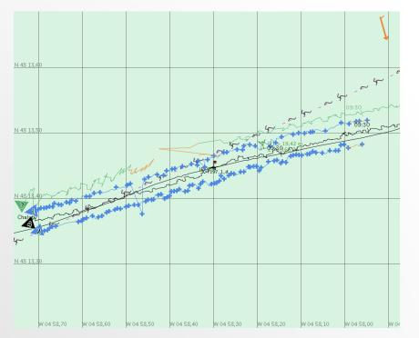
During this test the Marport Positioning System is compared in realtime to the SONARDYNE SCOUT Positioning System. The Marport beacons are marked 1, 2.
